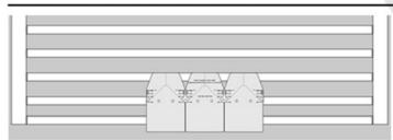
When laying the Speedy Tile, start in the middle of the roof and work outwards. Work from one side across if the roof facet has a verge at one end and a ridge at the other end. Working from the bottom on the starter course then build upwards
